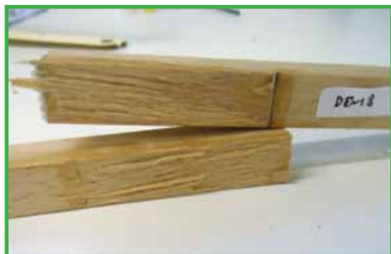
Left: Finding the optimum attributes for new 4 Minute Speed Epoxy II Above: Using hard wood to test pieces with different ratio epoxy mixes.
