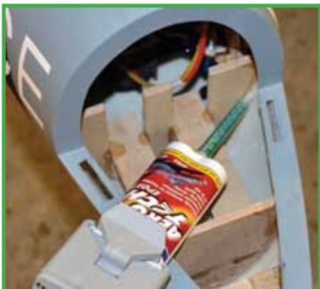
Aero Tech epoxy was developed for areas such as formers in glass composites fuselages.
