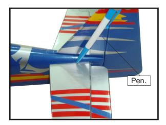
☐ 4) Remove the stabilizer. Using a modeling knife, remove the covering from below the lines you drew.
