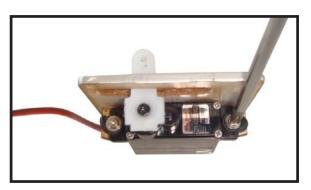
7) Apply 1-2 drops of thin C/A to each of the mounting tabs. Allow the C/A to cure without using accelerator.
