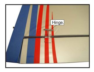
☐ 4) Deflect the aileron and completely saturate each hinge with thin C/A glue. The ailerons front surface should lightly contact the wing during this procedure. Ideally, when thehinges are glued in place, a 1/64" gap or less will be maintained throughout the lengh of the aileron to the wing panel hinge line.
