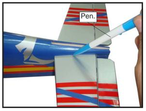
☐ 7) Remove the stabilizer. Using the lines you just drew as a guide, carefully remove the covering from between them using a modeling knife.
