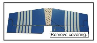
When cutting through the covering to remove it, cut with only enough pressure to only cut through the covering itself. Cutting into the balsa structure may weaken it.
