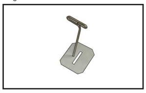
☐ 2) Remove each hinge from the wing panel and aileron and place a T-pin in the center of each hinge. Slide each hinge into the aileron until the T-pin is snug against the aileron. This will help ensure an equal amount of hinge is on either side of the hinge line when the aileron is mounted to the wing panel.
