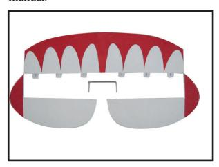
2) Carefully remove the elevator from one of the horizontal stabilizer panels. Note the position of the hinges. Used C/A glue to fix the hinges position.
