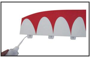
3) Remove each hinge from the horizontal stabilizer panel and elevator and place a Tpin in the center of each hunge. Slide each hinge into the elevator until the T-pin is snug against the elevator. This will help ensure an equal amount of hinge is on either side of the hinge line when the elevator is mounted to the horizontal stabilizer panel.
