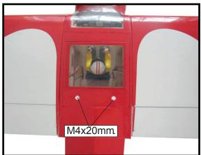
INSTALLATION STRUT WING -FUSELAGE.
