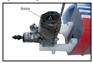
3) Use a drill to drill the four holes in the engine mount rails.
