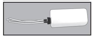
You should mark which tube is the vent and which is the fuel pickup when you attach fuel tubing to the tubes in the stopper. Once the tank is installed inside the fuselage, it may be difficult to determine which.
