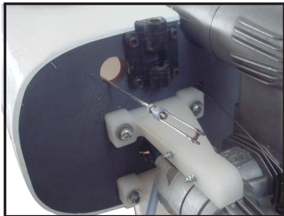
2) Install landing gear at the top Fuselage.
