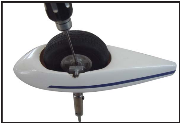
2) Install landing gear at the top Fuselage.
