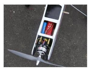
Ready to go. This photo (left) shows the hatch open shows some of the layout. Taped beside the motor is the RPM sensor of the datalogger. The LiPo is the red block seen through the hatch, the blue block is the 6v Rx battery. On the other side of the LiPo is the Opto ESC.
