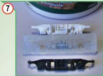
Create and Shape can replicate quite complex shapes such as this bogie frame using a mould made from silicone bath caul. Anthracite coal will give an excellent, small scale rock strata effect. Neat washing up liquid is a great release agent.
