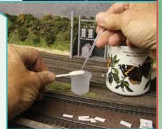
Use the pipette to dispense about a millilitre of Track Magic onto the swab to moisten.
